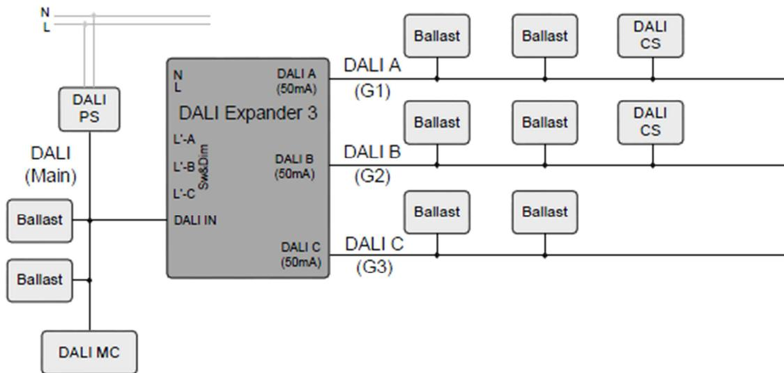
DALI input circuit available (separate DALI PS required). Control of DALI-sublines via short addresses from the DALI-Main-circuit or with the help of controls (e.g. DALI CS) in the output circuits
