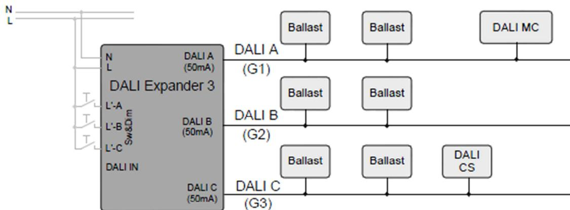
Stand Alone solution without DALI-circuit at the input. Control of the DALI output lines with Switch&Dim inputs or with controls in the output circuits (e.g. DALI MC or DALI CS) – if the DALI CS sends control commands to Group 5, per factory default line A and line C will receive this command broadcast
