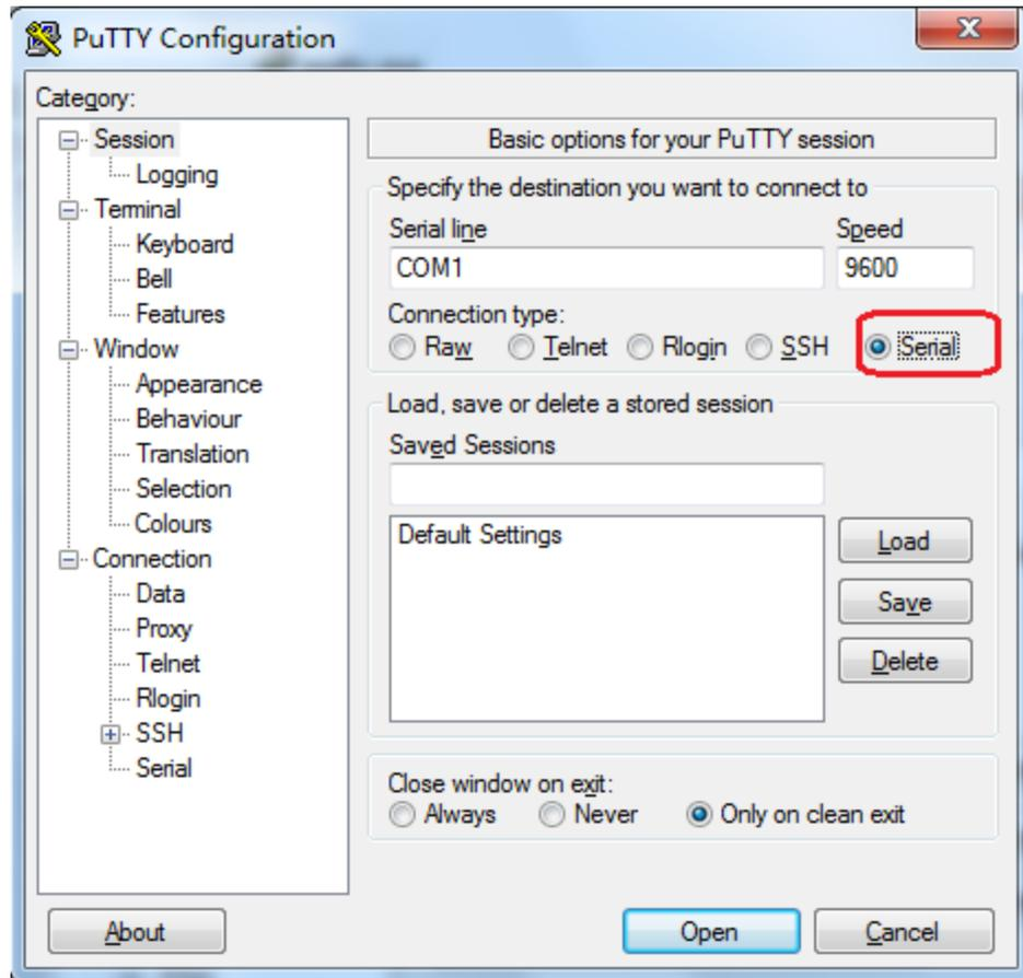
Select “Serial” node on the left tree, and configure the parameters of the serial port on the right window: **9600** bps, **8** bits, **None** parity, **1** stop bit and **None** flow control. And then open the putty serial communication window by click “open” button.
