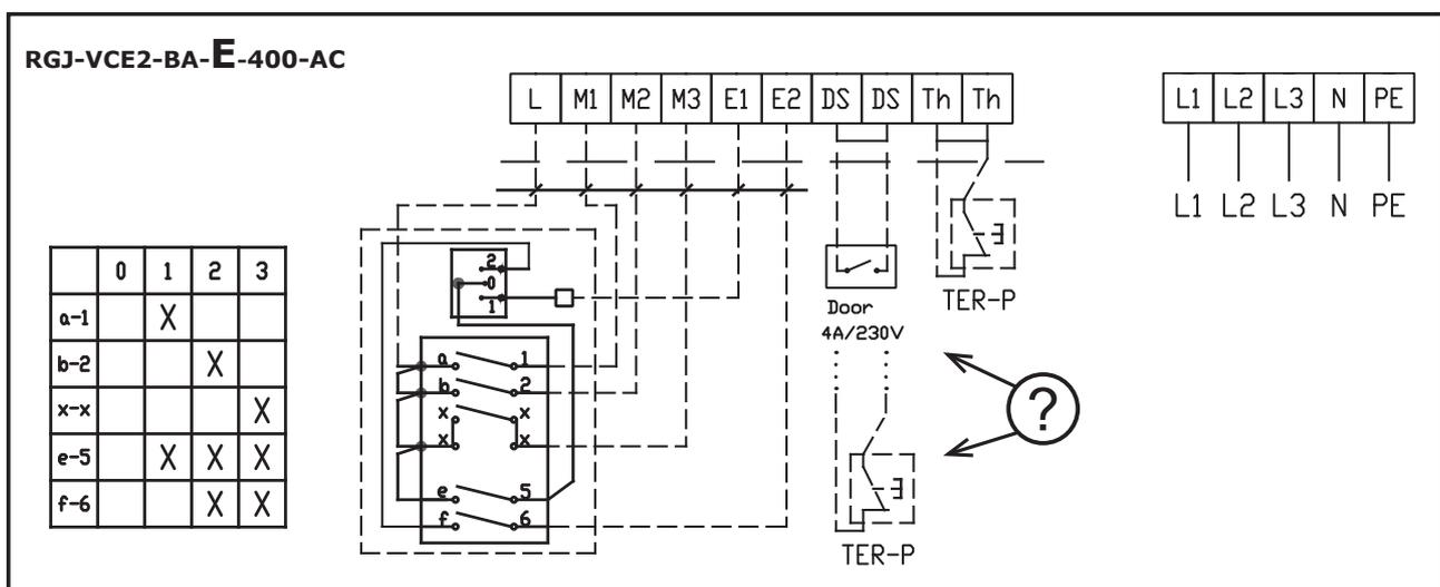
**\*A cable with a minimum cross-section of 6x0.5mm<sup>2</sup> is recommended for connecting the control.**
