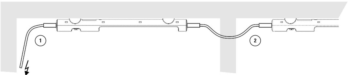
This illustration shows the LED 025 lamp in a daisy chain application. The lamps are conveniently connected via quick connection plugs – up to 10 lamps max. can be daisy-chained this way. The snap lock connectors ensure a stable electrical connection even if subjected to heavy vibration. The connection example shows a 230VAC application, using the following cables: connection cable with female connector, Art. No. 244356 (1); daisy chain extension cable with 2 connectors, Art. No. 244358 (2).
