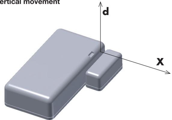
$X = 0 \text{ mm}$ , switching distance  $30 < d < 40 \text{ mm}$
