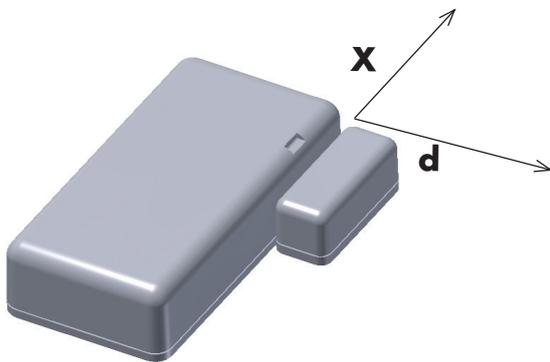
$X = +/- 5 \text{ mm}$ , switching distance  $20 \text{ mm} < d < 30 \text{ mm}$
