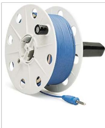
50 m measurement cable coiled onto a plastic drum. Connection to the inside end of the cable is made possible with a socket integrated into the drum. The other end is equipped with a banana plug. The drum axle with handle can be removed for space saving storage. Cable resistance can be compensated for with the rotary selector switch in the  $R_{LO}$  position.
