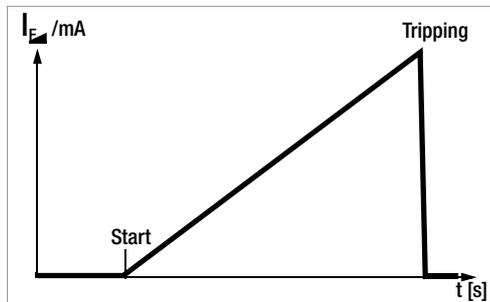
With the selector switch in the  $I_F$  position, slowly rising current flows via N and PE. The momentary measured current value is continuously displayed. When the RCCB is tripped, the last measured current value is displayed. A greatly reduced rate of increase is used for delayed RCCBs (type **S**).
