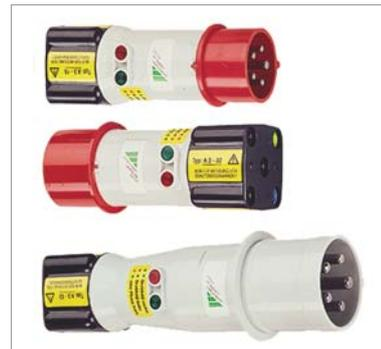
A3-16, A3-32 and A3-63 3-phase adapters are used for trouble-free connection of test instruments to 5-pole CEE outlets. The three variants differ with regard to plug size, which corresponds respectively to 5-pole CEE outlets with current ratings of 16, 32 and 63 A. Phase sequence is indicated with lamps at all three variants. Testing the effectiveness of safety
