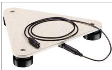
The 1081 floor probe makes it possible to measure the resistance of insulating floors in accordance with DIN VDE 0100-600, and EN 1081.
