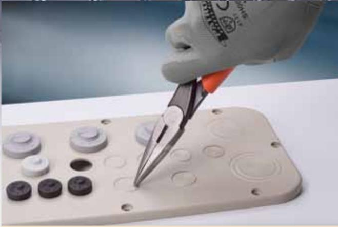
Make appropriate size hole to blind plate or knock-out plate. Avoid rough and sharp edges.
