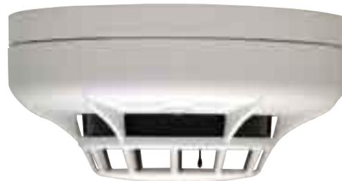
The ECO1003 photoelectric smoke detector's chamber has been specifically designed to be highly tolerant to the long term build-up of dust and other airborne contaminants. This high level of immunity significantly reduces the potential for unwanted alarms caused by settled dust increasing the detector's sensitivity. Additional immunity to unwanted alarms arising from short-lived transients is also provided through the use of special signal processing.
