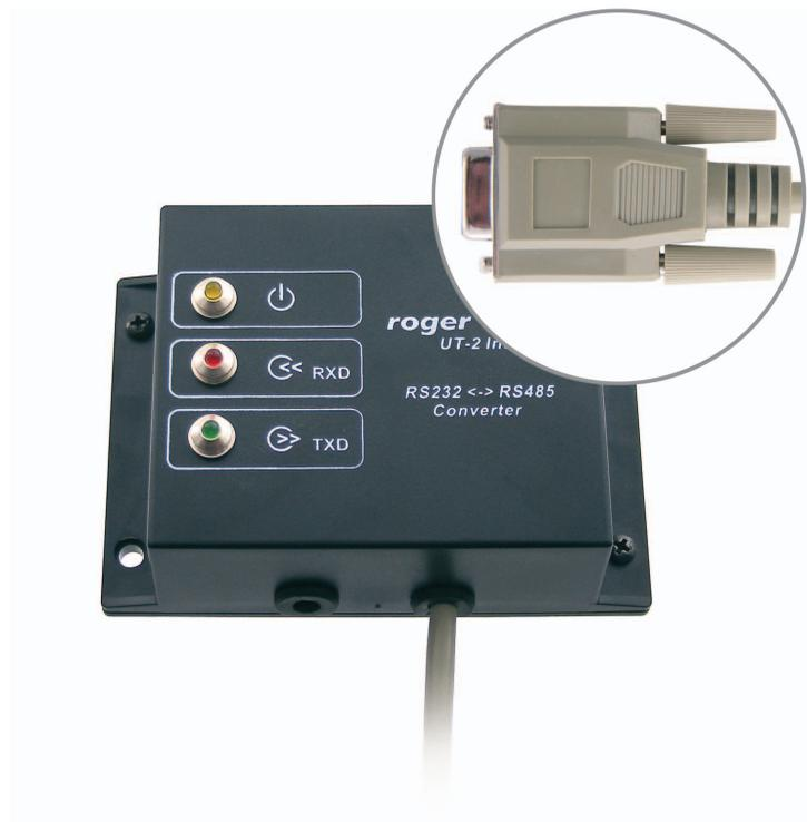
The UT-2 operates as an electrical converter between RS232 and RS485 communication interfaces. It can be used for programming of single access controller or the whole network (subsystem) of access controllers connected RS485 bus. UT-2 device enables bidirectional data transmission between access control devices and management software installed at PC.
