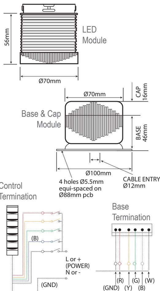
Termination to the 'B' Contact Controls a Blue LED and/or an Audible Module
