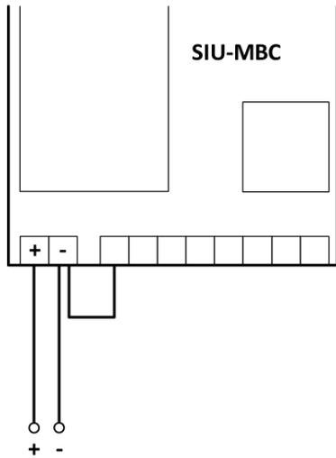
Connection of two devices and anti-fraud cables
