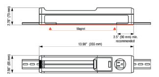
In plastic, aluminum or stainless steel cabinets the light can be mounted using screws together with inserted 35mm DIN rail sections. The drawing shows mounting on two 7 inch long pieces of 35mm DIN rail.
