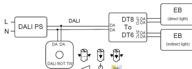
Application: balance- and level control of direct and indirect lighting with the help of a DT8toDT6 converter
