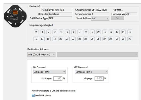
An additional feature is switching on by rotation (without pressing the button). This feature can be deactivated.
