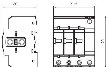
Application: Equipotential bonding in buildings, even those with external lightning protection of class III and IV, and in standard distributor housings.
