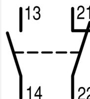
Contact travel diagram, stroke in connection with front element
