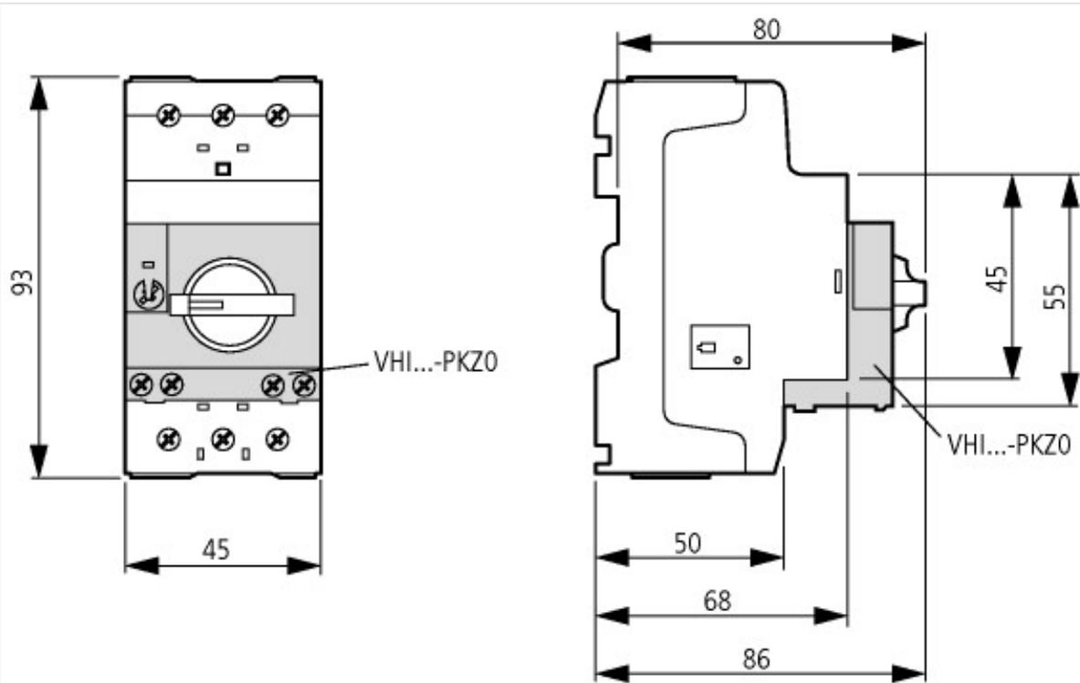
Motor-protective circuit-breakers with early-make auxiliary contacts
