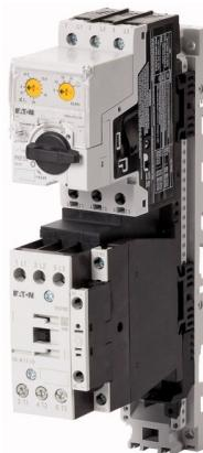
DOL starter, 380 V 400 V 415 V: 11 kW,  $I_q = 100$  kA,  $I_r = 8 - 32$  A, 24 V DC, DC voltage
