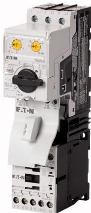
DOL starter, 380 V 400 V 415 V: 0.37 kW,  $I_q = 100$  kA,  $I_r = 0.3 - 1.2$  A, 230 V 50 Hz, 240 V 60 Hz, AC voltage
