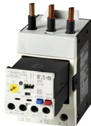
Overload relay, Direct mounting, Earth-fault protection: with,  $I_r = 20 - 100$  A, 1 N/O, 1 N/C
