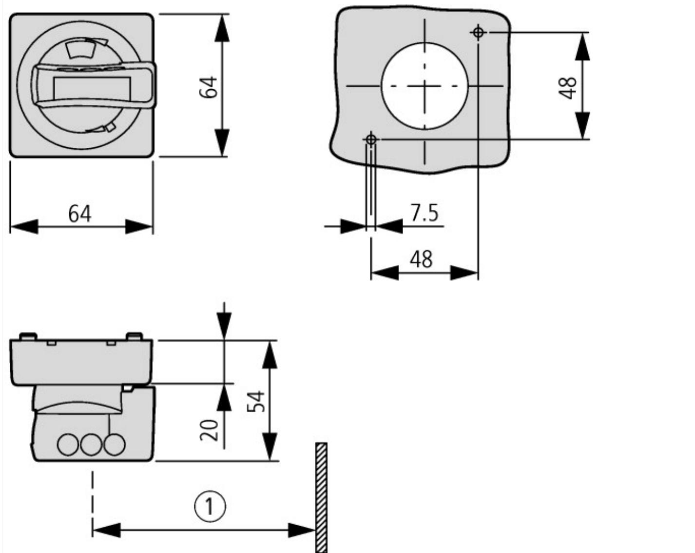
Mounting depth: 152 to 267 mm from the top edge of the top-hat rail to the front edge of the cabinet door/cover
