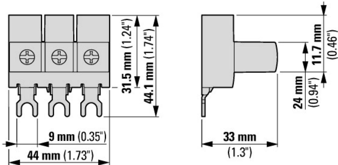
Overlapping mounting to extend the three-phase common link
