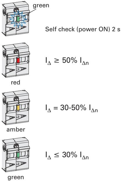
**Service Mode (measuring of residual current  $I_{\Delta}$ )**
