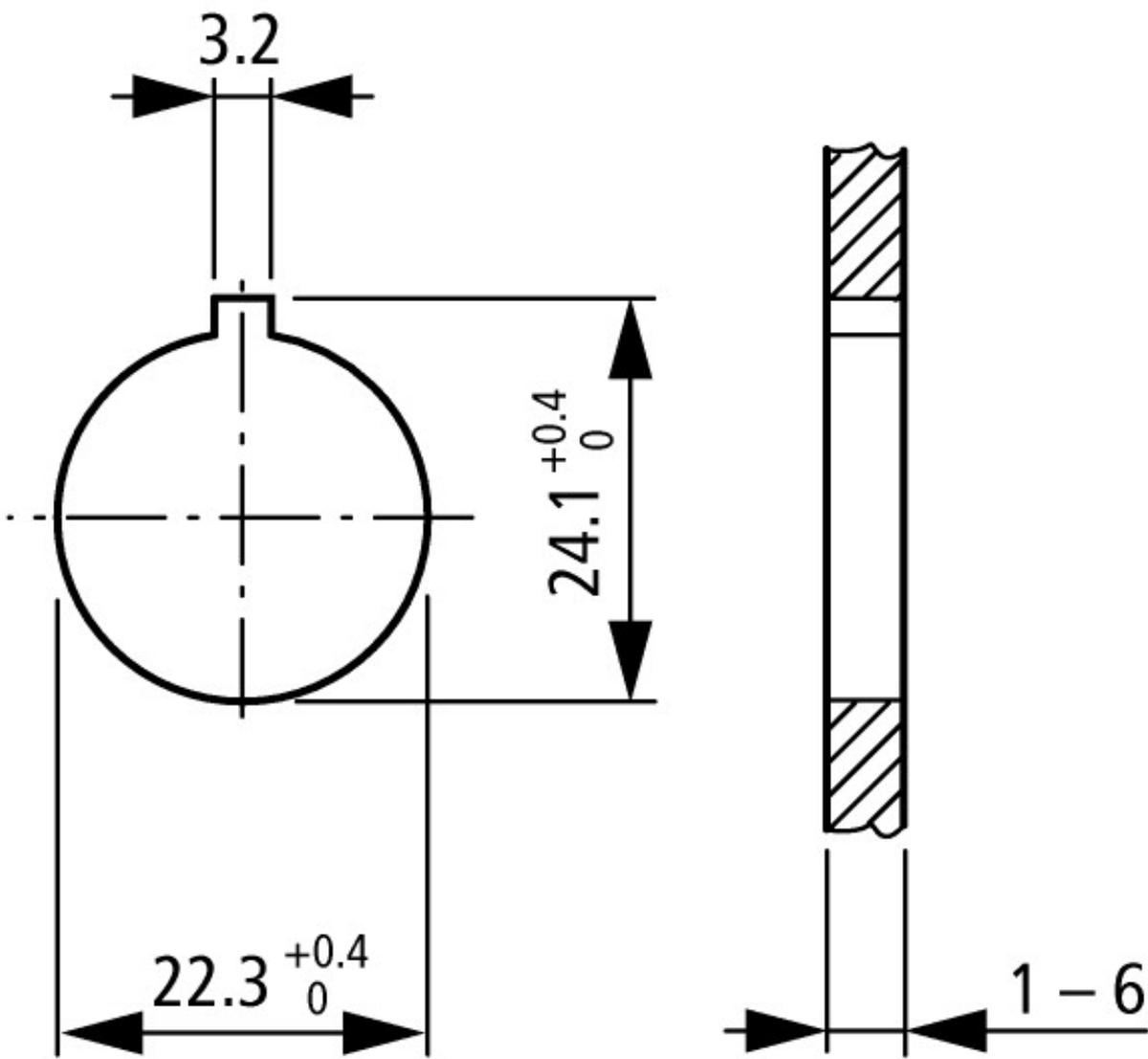
Mounting hole with lug slot
