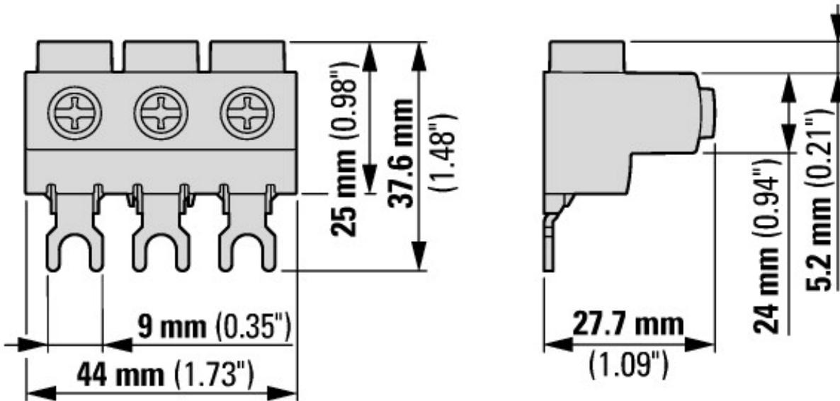
Overlapping mounting to extend the three-phase commoning link
