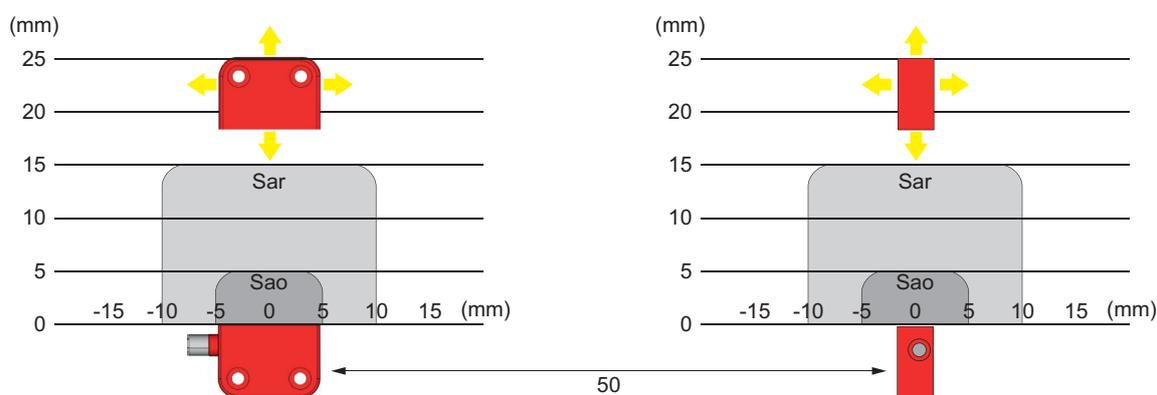
Note: the typical detection characteristic shown may vary from sensor to sensor.
