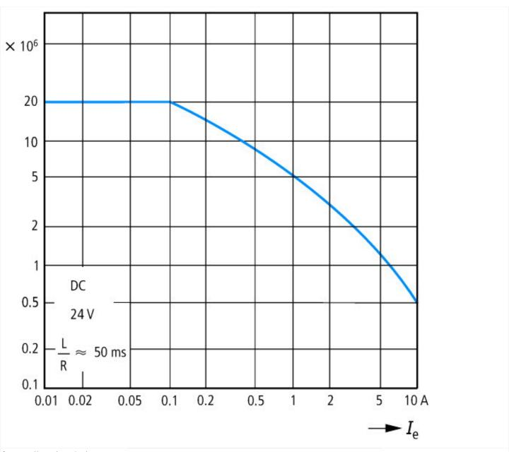
Component lifespan (operations)  $I_e$  = rated operational current
