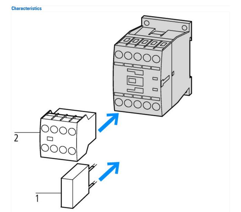
1: Suppressor 2: Auxiliary contact module
