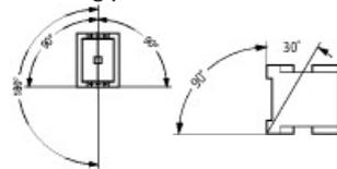
Mechanical shock resistance (IEC/EN 60068-2-27)
