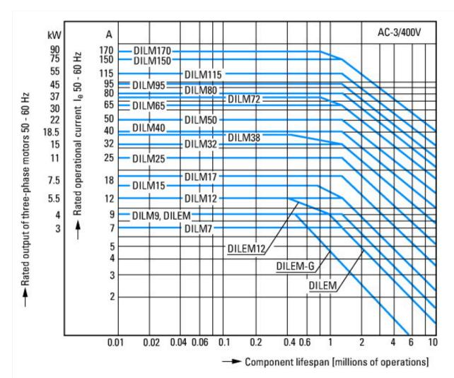
Squirrel-cage motor Operating characteristics Starting:from rest Stopping:after attaining full running speed Electrical characteristics Make: up to 6 x rated motor current Break: up to 1 x rated motor current Utilization category 100 % AC-3 Typical applications
