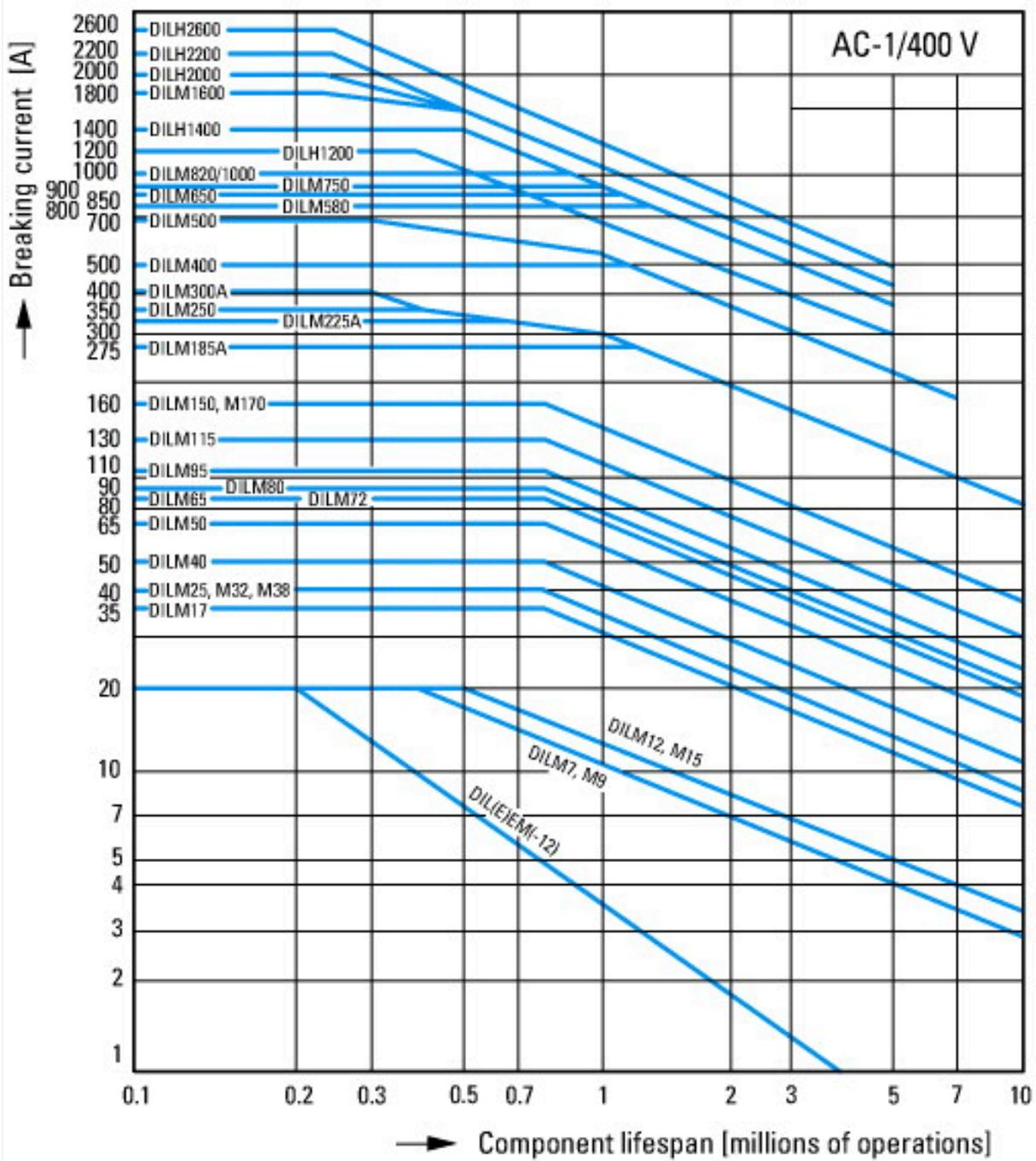
Switching duty for non-motor loads, 3-pole, 4-pole
