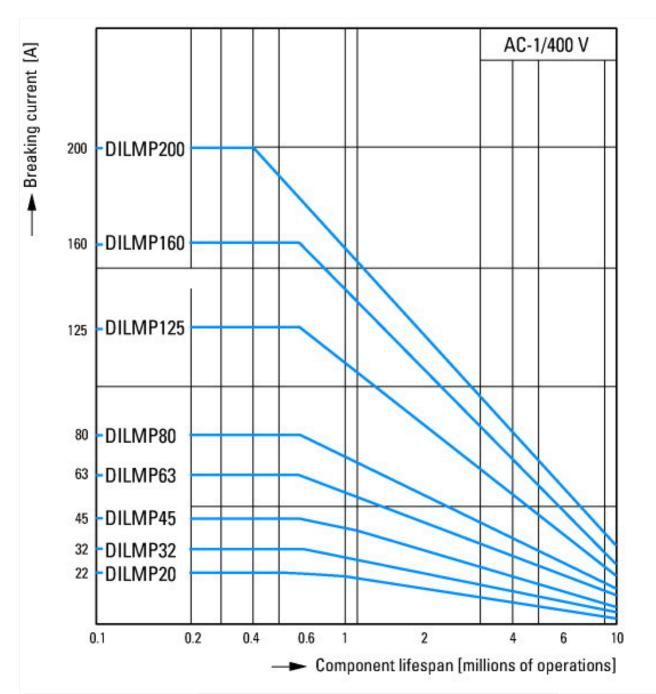
Switching conditions for 4 pole, non-motor loads Operating characteristics
