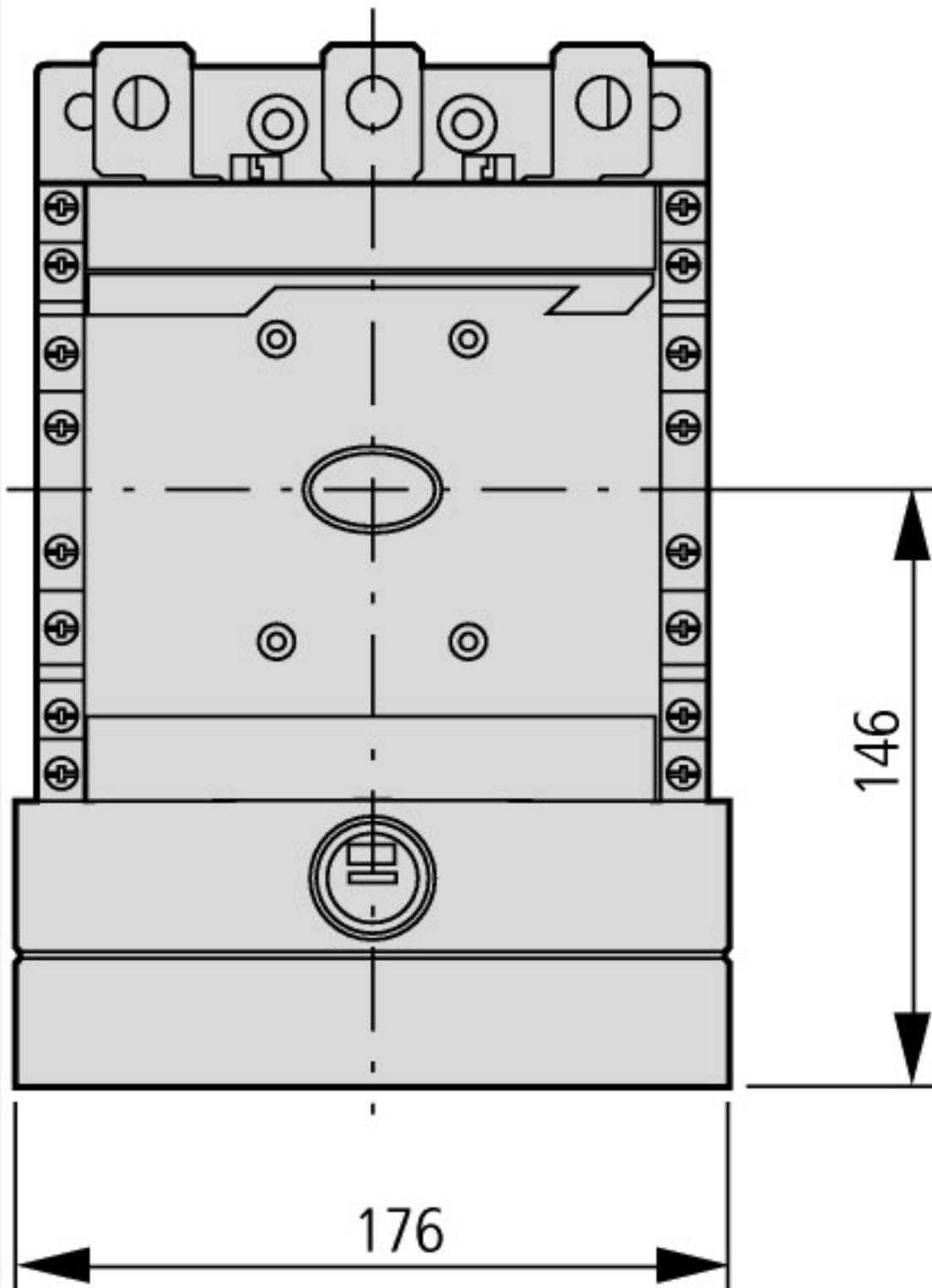
Contacter with star-point bridge and terminal shroud
