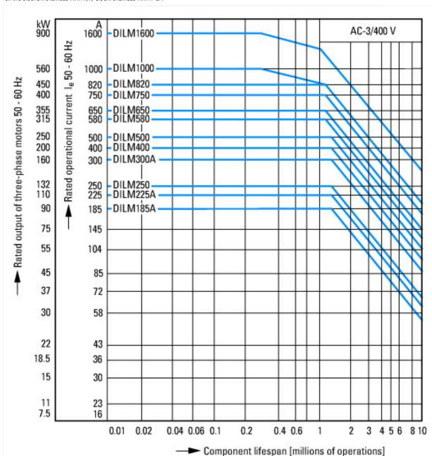
Normal AC induction motor Operating characteristics Switch on: from stop Switch off: during run Electrical characteristics: Switch on: up to 6 x Rated motor current Switch off: up to 1 x Rated motor current Utility category 100 % AC-3 Typical Applications Compressors Lifts Mixers Pumps Escalators Agitators fan Conveyor belts Centrifuges Hinged flaps Bucket-elevator
