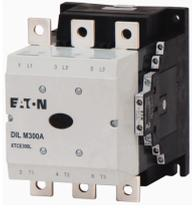
**Contactors, 380 V 400 V 160 kW, 2 N/O, 2 NC, RDC 48: 24 - 48 V DC, DC operation, Screw connection**
