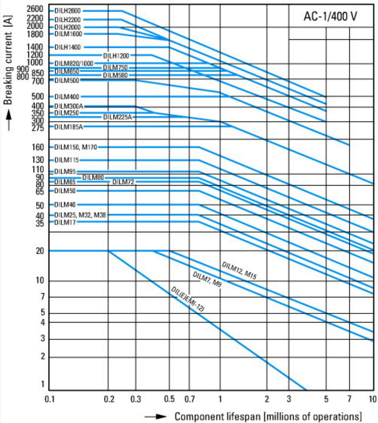
Switching conditions for 3 pole, non-motor loads
