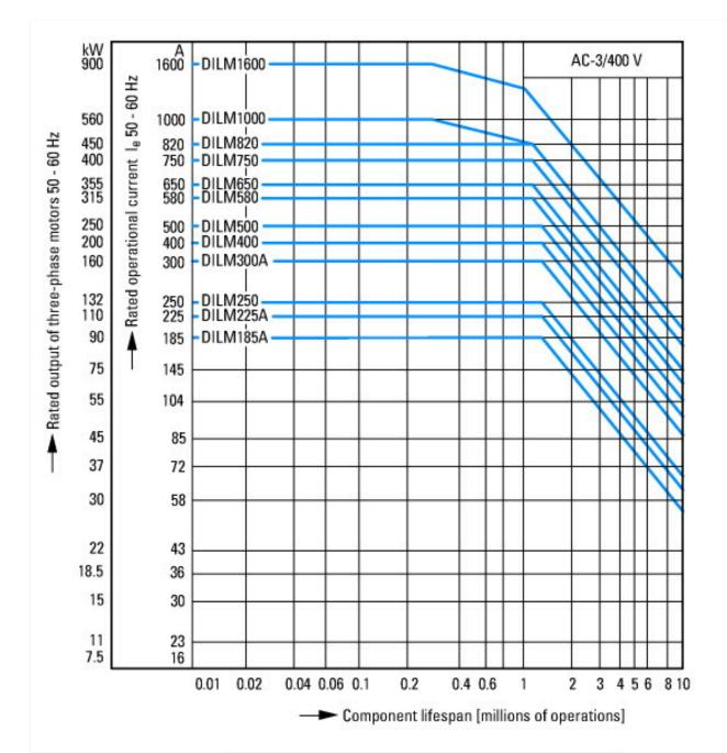
Normal switching duty Normal AC induction motor Operating characteristics Switch on: from stop Switch off: during run Electrical characteristics: Switch on: up to 6 x Rated motor current Switch off: up to 1 x Rated motor current Utility category 100 % AC-3 **Typical Applications** Compressors Mixers Pumps Escalators Agitators fan Conveyor belts Centrifuges Hinged flaps
