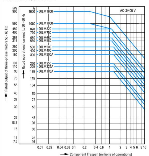
Normal AC induction motor Operating characteristics Switch on: from stop Switch off: during run Electrical characteristics: Switch on: up to 6 x Rated motor current Switch off: up to 1 x Rated motor current Utility category 100 % AC-3 Typical Applications Compressors Lifts Mixers Pumps Escalators Agitators fan Conveyor belts Centrifuges Hinged flaps Bucket-elevator Air-conditioning systems
