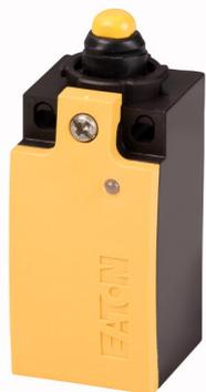
**Safety position switch, LSE, Position switch with electronically adjustable operating point, Basic device, expandable, 1 N/O, 1 NC, Yellow, Insulated material, Cage Clamp, -25 - +70 °C**
