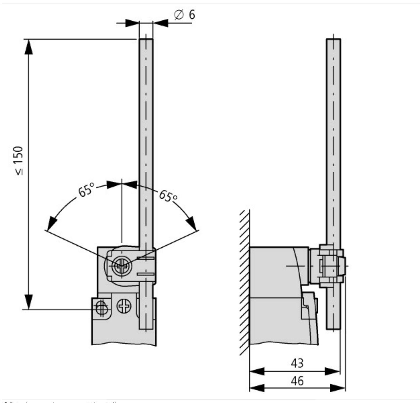
① Tightening torque of cover screws: 0.8 Nm  $\pm 0.2$  Nm
