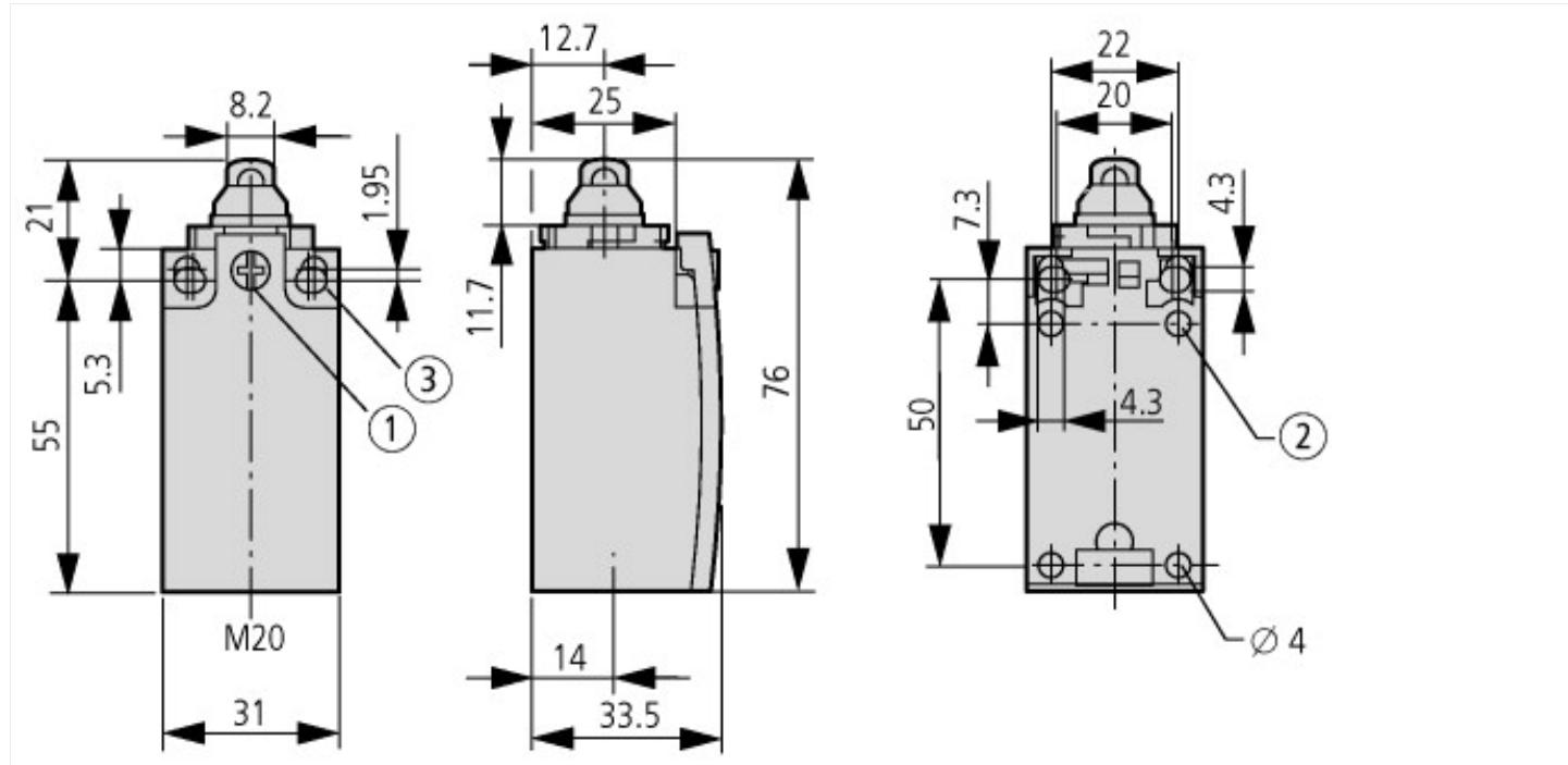
① Tightening torque of cover screws:  $0.8 \text{ Nm} \pm 0.2 \text{ Nm}$
