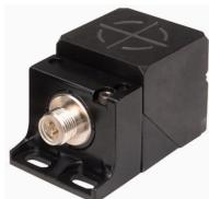
Proximity switch, inductive, 1N/O+1N/C, Sn=20mm, 4L, 10-48VDC, NPN, PNP, quad.40, insulated material
