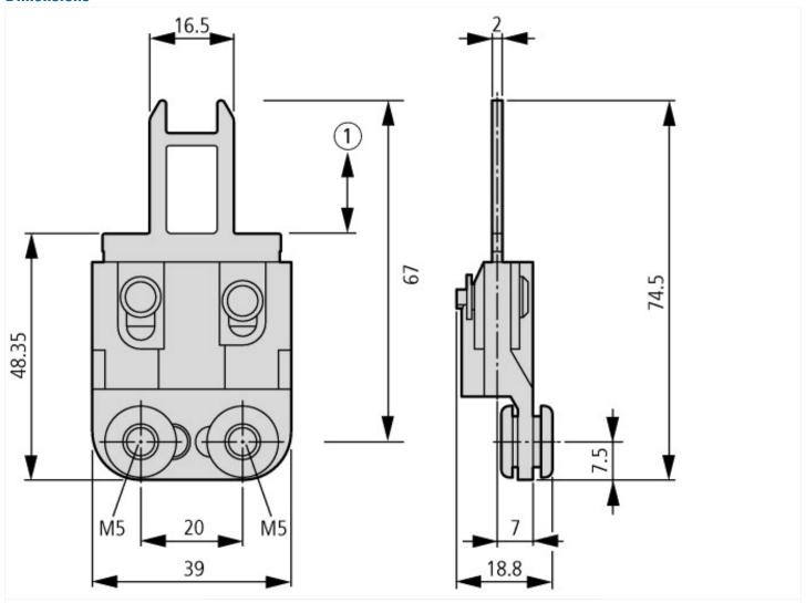
Fixing only allowed with M5 fixing screw and washer according to DIN EN ISO 7093  $\stackrel{\frown}{0}$  Distance to device head = 0.1  $\dots$  3.0 mm
