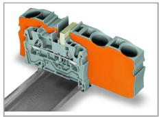
Step-down jumpers may common terminal blocks of different sizes, without losing a conductor clamping point. This can be beneficial on long conductor runs where voltage drops may be problematic. A large conductor can be easily connected to smaller conductors at the distribution point.
