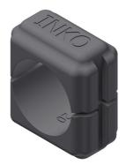
**Additional information:** For Module base units from 6 to 20 mm tubing: Position the first half part of the tube clamp into the steel module base before placing the tubing. Add the second half part and a Pressure Plate before fixing with the Lock Plate. To add an additional level to the module: Release the Lock Plate and remove the Pressure Plate on top of the clamp halves surrounding the tubing. Place a single bolted module base where the Pressure Plate was and retighten using the Lock Plate.
