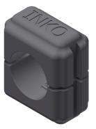
**Additional information:** For Module base units from 6 to 20 mm tubing: Position the first half part of the tube clamp into the steel module base before placing the tubing. Add the second half part and a Pressure Plate before fixing with the Lock Plate. To add an additional level to the module: Release the Lock Plate and remove the Pressure Plate on top of the clamp halves surrounding the tubing. Place a single bolted module base where the Pressure Plate was and retighten using the Lock Plate.
