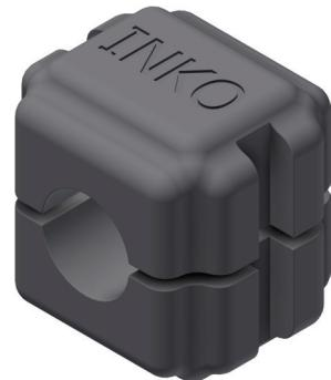
**Additional information:** For Module base units from 6 to 20 mm tubing: Position the first half part of the tube clamp into the steel module base before placing the tubing. Add the second half part and a Pressure Plate before fixing with the Lock Plate. To add an additional level to the module: Release the Lock Plate and remove the Pressure Plate on top of the clamp halves surrounding the tubing. Place a single bolted module base where the Pressure Plate was and retighten using the Lock Plate.
