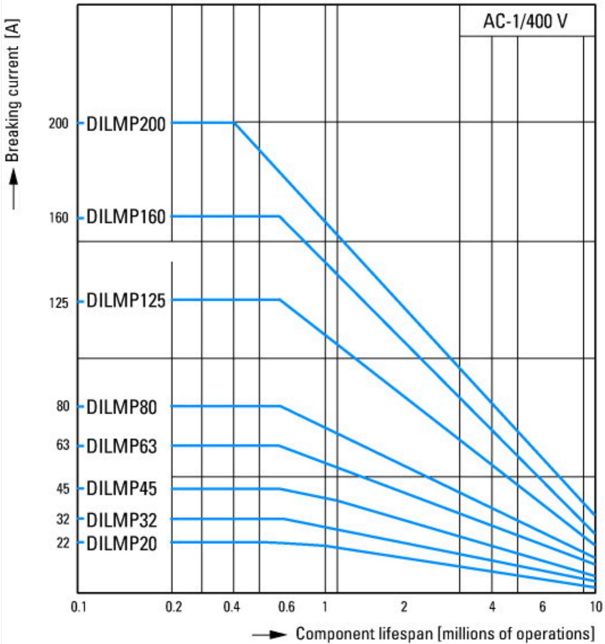
Switching conditions for 4 pole, non-motor loads
