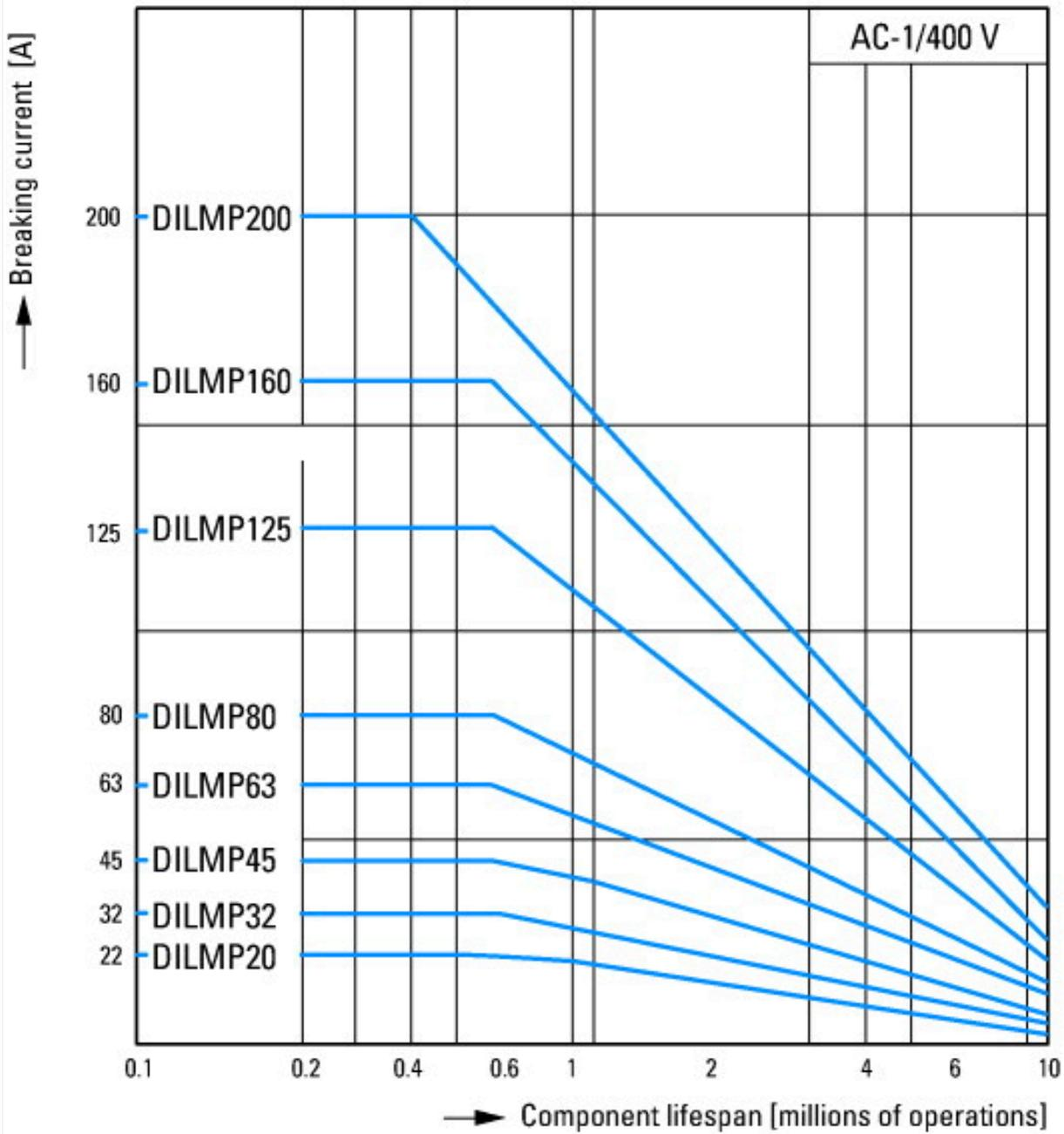
Switching conditions for 4 pole, non-motor loads
