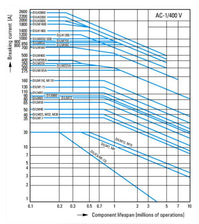
Switching conditions for non-motor consumers, 3 pole, 4 pole Operating characteristics Non inductive and slightly inductive loads Electrical characteristics
