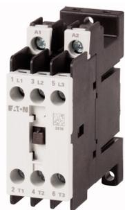
**Contactor relay, 24 V DC, N/O = Normally open: 1 N/O, N/C = Normally closed: 2 NC, Screw terminals, DC operation**
