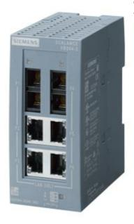
SCALANCE XB004-2 unmanaged Industrial Ethernet Switch for 10/100 Mbit/s; for setting up small star and line topologies; LED diagnostics, IP20, 24V DC power supply, with 4x 10/100 Mbit/s twisted pair ports with RJ45 sockets; 2x 100 Mbit/s multimode glass FOC port with SC socket; Manual available as a download
