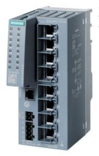
SCALANCE XC208 managed Layer 2 IE switch; IEC 62443-4-2 certified; 8x 10/100 Mbps RJ45 ports; 1x console port; diagnostics LED; redundant power supply; temp. range -40 °C to +70 °C; mounting: DIN rail/S7 mounting rail/wall Office redundancy functions features (RSTP, VLAN,...); PROFINET IO device Ethernet/IPcompliant C-plug slot;
